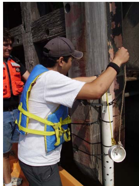
Figure 2.5 PVC tube for YSI unit, Site 2.
