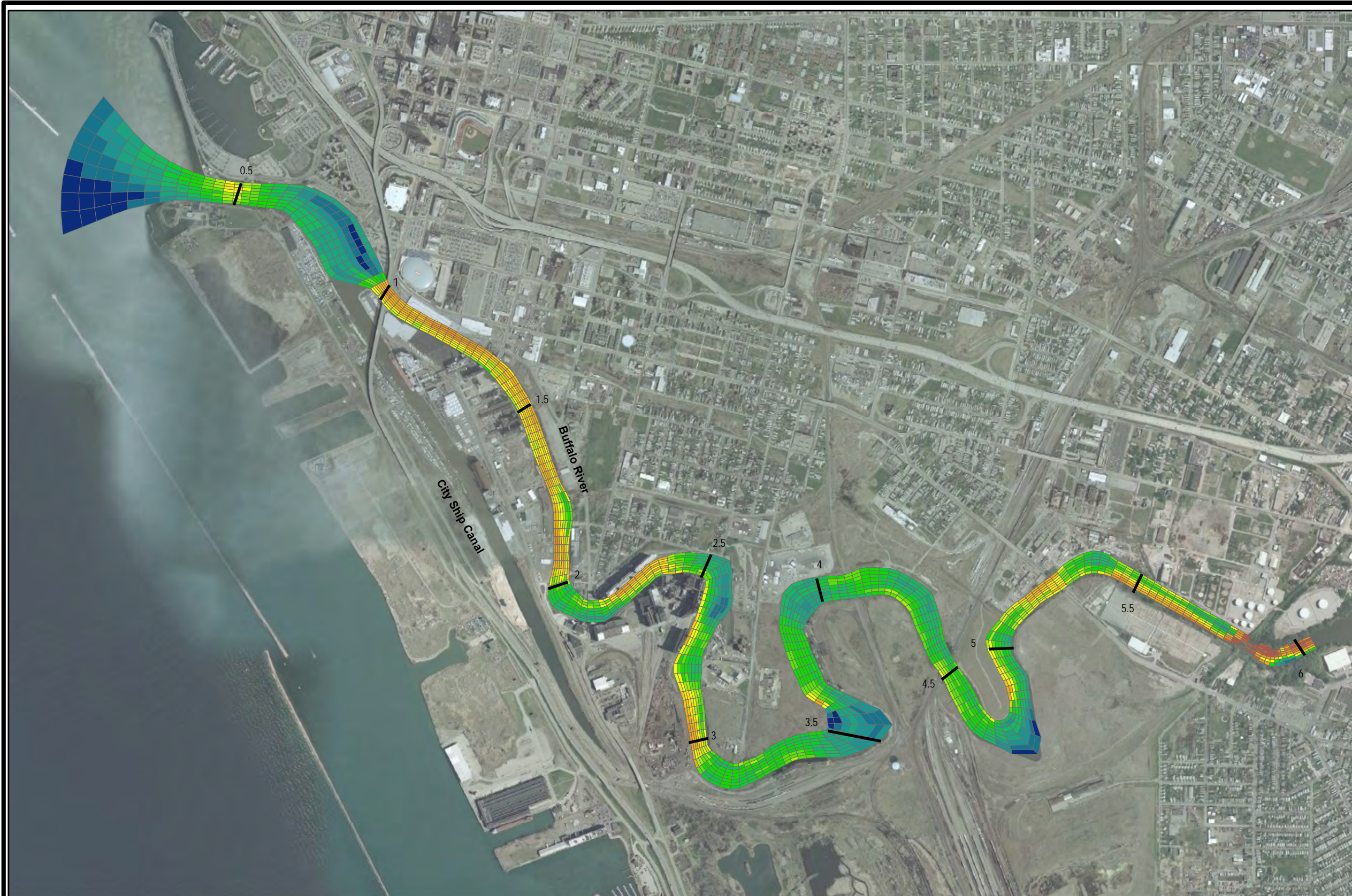
Buffalo River Model Predicted Bottom Shear Stress at the Peak of the January 29, 2002 High Flow Event (10-year Recurrence Interval)
