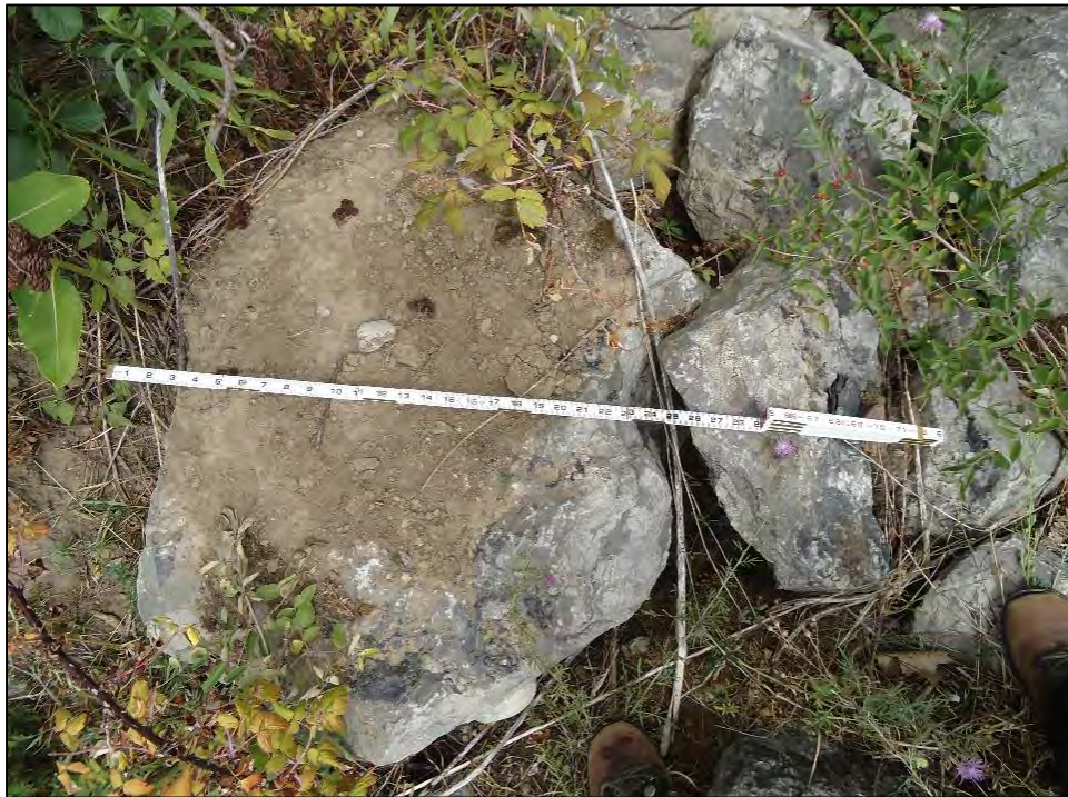
Figure 3.1.1-2. Typical Rip-rap Stone Sizes in Sampling Quadrats
