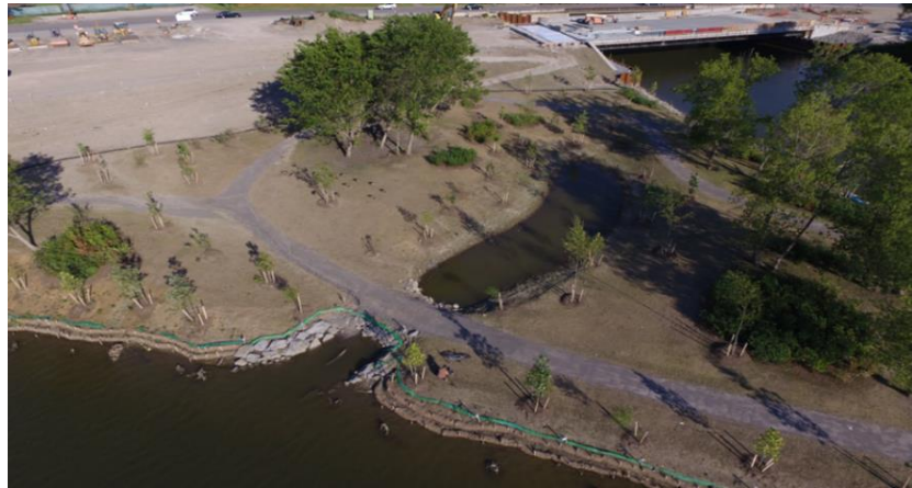
Figure 8. The Bailey Avenue habitat restoration site identified in the Habitat Action Plan. This site restores approximately 765 linear feet of shoreline and the inlet opens up additional fish habitat. Taken from ECDEP, 2017.
